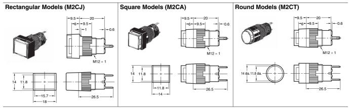
Note: Unless specified, there is a tolerance of  $\pm 0.4$  mm for dimensions.
