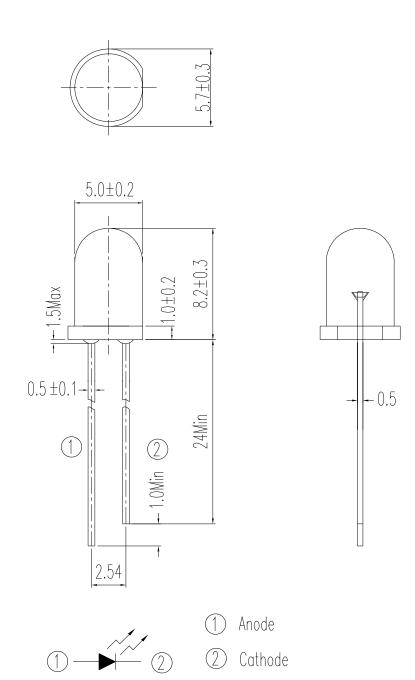
Note: Tolerances unless dimensions ±0.25mm
