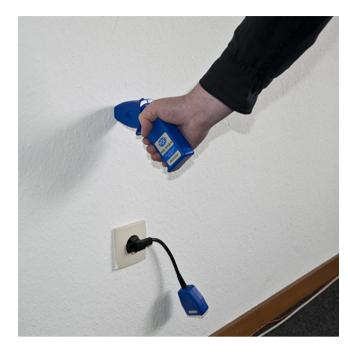
PCE-191 CB is a handheld, portable wire tracer, cable detector or cable fault meter used for locating wires and cables hidden behind walls and insulation. Comprised of a signal transmitter and receiver, this easy-to-use cable locating device emits an acoustic alarm.
