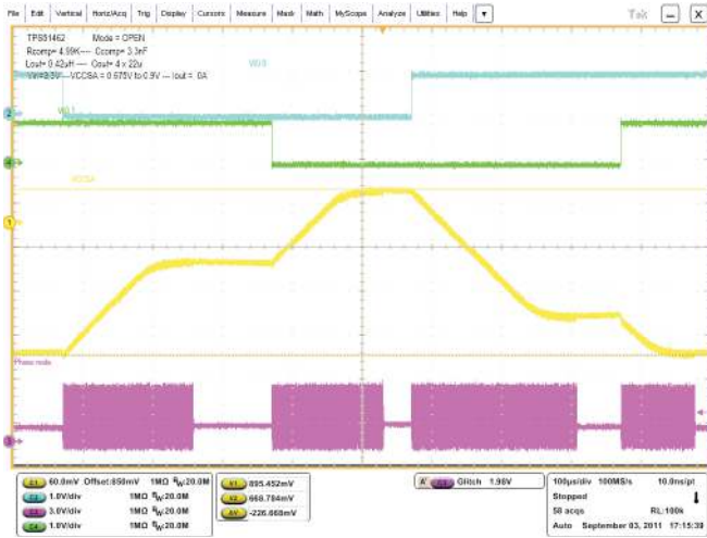
Figure 14. Mode=8, I OUT = 0 A, VID Transitions
