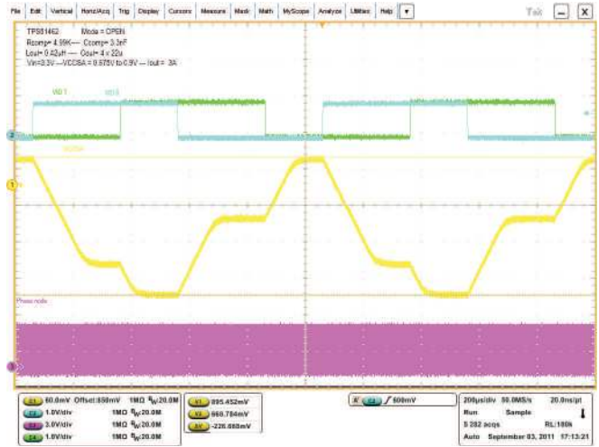
Figure 15. Mode=8, I OUT = 3 A, VID Transitions
