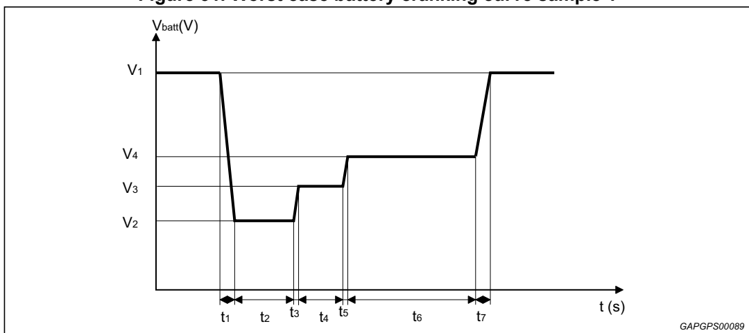
Figure 31. Worst case battery cranking curve sample 1
