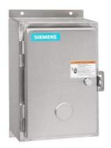
Non-reversing NEMA contactor, Size 0, Three phase full voltage, Contactor amp rating 18A, 3 wire (NO aux included), 110V 50Hz / 120V 60Hz coil, Non-combination type, Encl NEMA type 4X 304 S-Steel, Water/dust tight noncorrosive, Standard width enclosure
