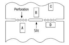
\*1 A > D is valid when stress is added vertically to the perforation as with Hand Separation.If a Cutting Disc is used, stress will be diagonal to the PCB, therefore A > D is invalid.
