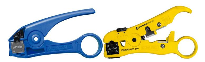
The **UST-135** tool strips RG7 & RG11. The blade UST-235 can be used on 2 sides. One side of the cassette has a strip-stop for consistent strip length.
