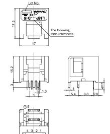
Terminal number 1 - Vcc 2 GND 3 + Vcc4 OUT 5 + IN 6 - IN Current
