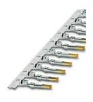
Crimp contact, Socket, rolled, Taped articles, number of pieces per reel: 500, contact diameter: 1 mm, crimp range: 0.22 mm² ... 0.56 mm², Item is lead-free in accordance with RoHS II without Exemption 6c (Pb <0.1%)
