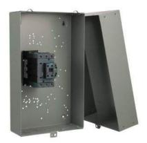
Electrically held lighting contactor, Contactor amp rating 100A, 0 N.C. / 3 N.O. Poles, 208VAC 50/60HZ coil, 1 NO / 1 NC auxiliary contacts Non-combination type, (no disconnect device), Enclosure NEMA type 1, Indoor general purpose use
