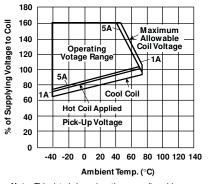
Note: This data is based on the max. allow able temperature for E type insulation coil (115°C).
