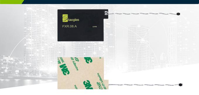
The FXR.08.52.0075X.A is a rectangular, flexible, NFC (Near Field Communications) antenna for use in mobile devices and other applications such as keycards, payment systems, and boarding passes. The design provides a flexible NFC antenna with 75mm twisted pair 28AWG cable that can be adhered to the plastic enclosure of the device for ease of installation and work with specific 13.56MHz RFID and NFC chips which need to connect via JST ACH connector.
