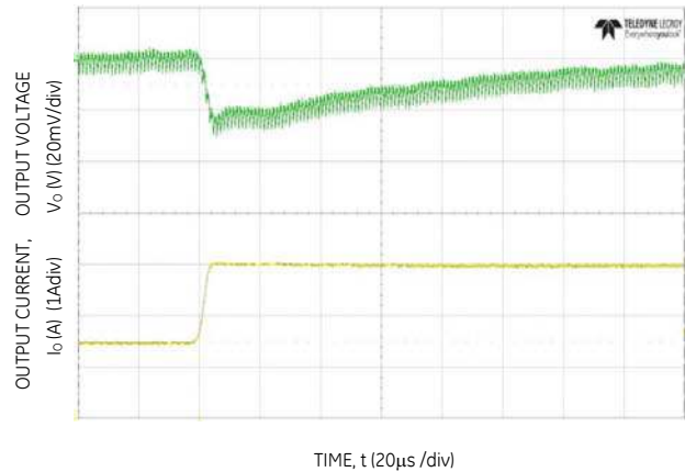
Figure 34. Transient Response to Dynamic Load Change from 50% to 100% at 12Vin, C_{out}=2 \times 47 \mu F + 1 \times 330 \mu F , C_{Tune}=2700pF , R_{Tune}=300\Omega
