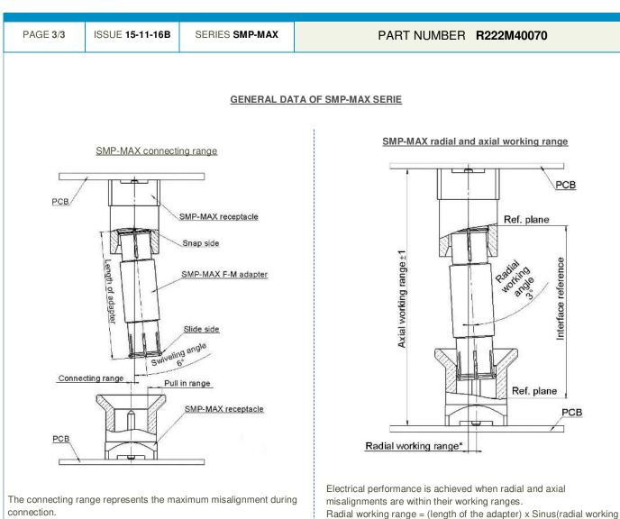
The swiveling angle is the maximum possible angle of the adapter in a snap receptacle.
