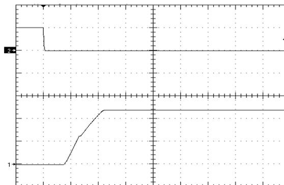
Figure 10. Startup Waveform via Enable Pin, time scale 10mS/div. Vin=Vin\_nom, full resistive load + 2200uF, Ch1=Ch2=5V/div (negative enable.)
