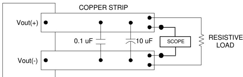
Note: Use a 0.1 $\mu$ F X7R ceramic capacitor and a 10 $\mu$ F @ 25V tantalum capacitor. Scope measurement should be made using a BNC socket. Position the load 3 in. [76mm] from module.
