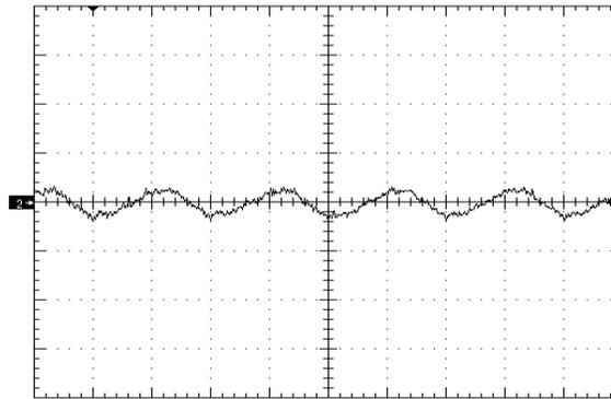
Figure 8. Input Reflected Ripple Current time scale - 1uS/div. Vin=Vin\_nom, full resistive load (10mA/div)
