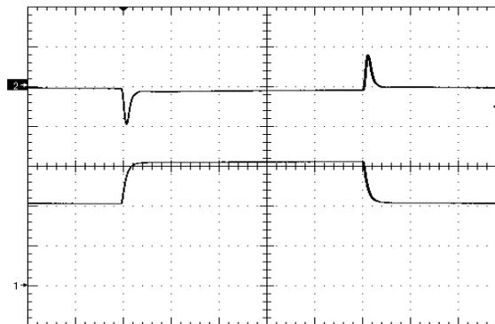
Figure 12. Load Transient Response (100mV/div), di/dt=0.1A/uS, 50% - 75% - 50% of full load, time scale: 200uS/div. Ch1 = 1A/div.
