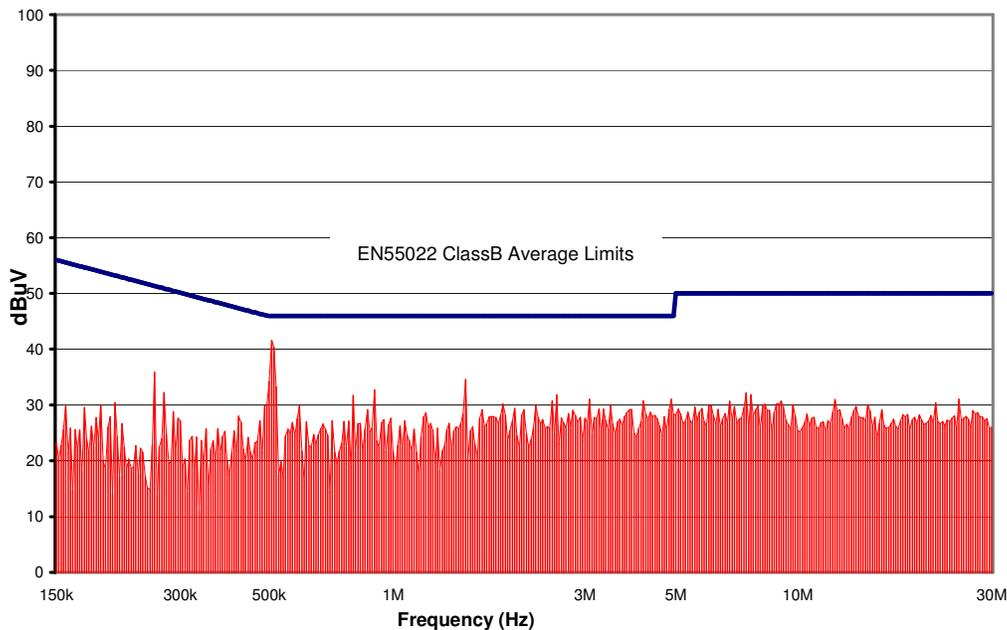
Figure 18. CPT4B36 Conducted Emissions using above specified input filter.
