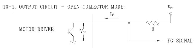
CAUTION: THE FG SINGAL LEAD WIRE MUST BE KEPT AWAY FROM "+" LEAD WIRE & "-" LEAD WIRE.
