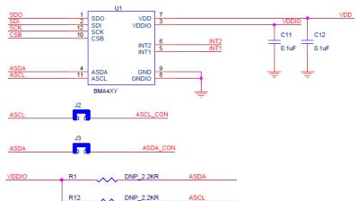
By default, ASDA and ASCL can be connected by PIN#8 and PIN#14. When J2 and J3 are removed, ASDA and ASCL are connected to VDDIO only.
