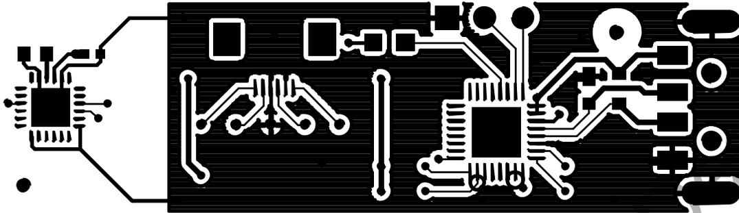
Figure 12. Si7005 Dongle Board Layout Top Layer
