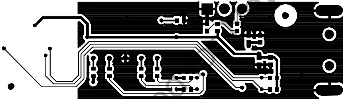
Figure 13. Si7005 Dongle Board Layout Bottom Layer
