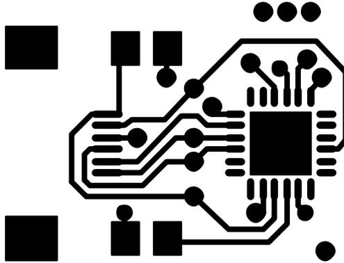
Figure 15. Si7005 Evaluation Board Layout Top Layer
