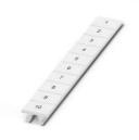
Zack marker strip, Strip, white, labeled, can be labeled with: CMS-P1-PLOTTER, Printed vertically: consecutive numbers 1  $\dots$  10, 11  $\dots$  20, etc. up to 91  $\dots$  100, mounting type: snapped, for terminal block width: 8.2 mm, lettering field size: 10. 5 x 8.15 mm, Number of individual labels: 10
