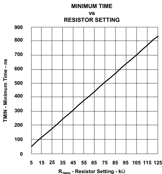
Figure 12. Minimum Time TMIN Over Setting Resistor R_{TMIN}
