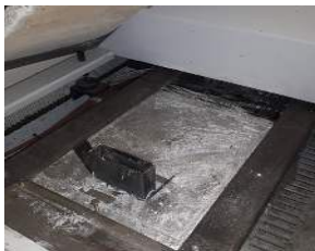
Wave solder pot with dross
