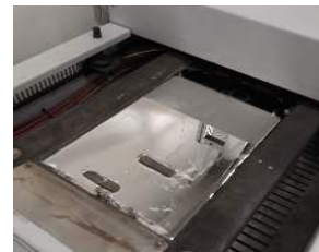
Solder pot post cleaning. Shiny with no evidence of dross.
