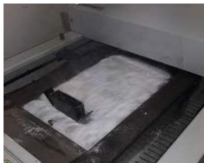
A thick layer of 5744 placed on top of solder surface.
