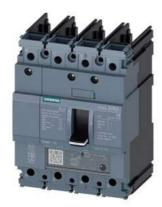
circuit breaker 3VA5 UL frame 125 breaking capacity class M 35kA @ 480 V 4-pole, line protection TM230, FTAM, In=90A overload protection Ir=90A fixed short-circuit protection Ii=5...10 x In N conductor protection 100% without connection
