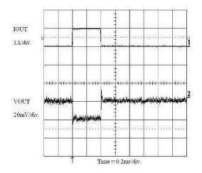
Figure 36. Load Transient Response (1 mA to 1 A) V<sub>IN</sub> = 2.2 V
