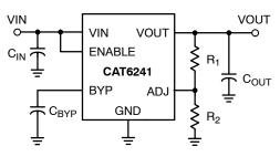
Figure 37. Adjustable Output Resistor Divider
