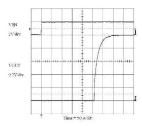
Figure 29. Enable Turn-on (1 mA Load)
