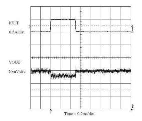
Figure 23. Load Transient Response (1 mA to 500 mA)  $V_{IN}$  = 2.0 V
