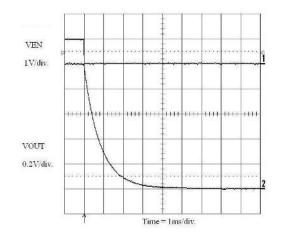
Figure 30. Enable Turn-off (1 mA Load)
