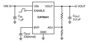
Figure 1. Application Schematic
