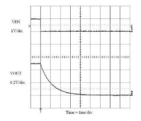
Figure 15. Enable Turn-off (1 mA Load)
