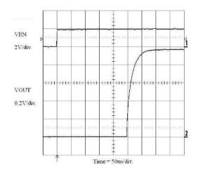
Figure 31. Enable Turn-on (1 A Load)
