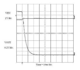
Figure 32. Enable Turn-off (1 A Load)
