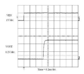
Figure 14. Enable Turn-on (1 mA Load)
