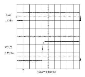
Figure 16. Enable Turn-on (350 mA Load)
