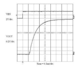
Figure 34. Enable Turn-on (1 A Load) C<sub>BYP</sub> = 470 pF
