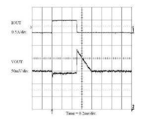
Figure 21. Load Transient Response (1 mA to 500 mA) V<sub>IN</sub> = 1.8 V
