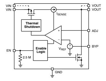
Figure 2. Simplified Block Diagram
