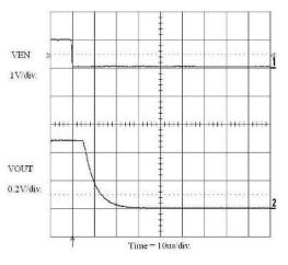
Figure 17. Enable Turn-off (350 mA Load)
