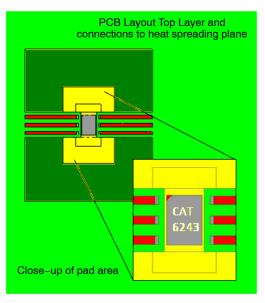
Figure 39. Topside Copper Foil Pattern for Heat Dissipation
