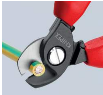
Cut performed with a Cable Shear: easy, clean cut without any deformation of the cable
