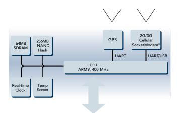
80 pin B2B connector Battery / GPIO / ADC / SPI / I2C / JTAG / Ethernet / USB Host / USB Device / GPS PPS - Data / Serial UARTs / LEDs
