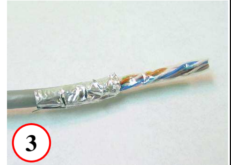
3 Fold back shield and drain wire
