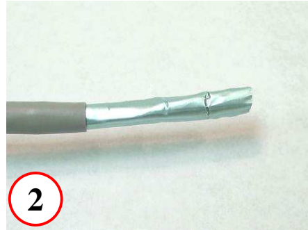
2 Trim off 1" to 2" of cable jacket
