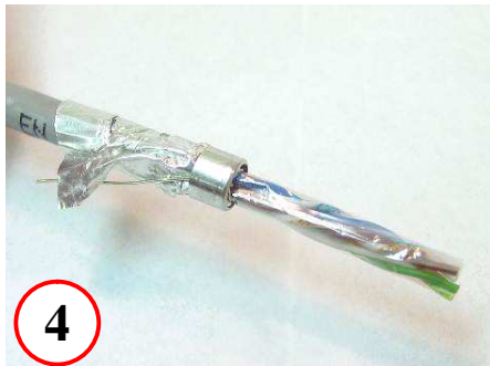
4 Slide ferrule over jacket and shield. Do not trap any insulation between shield and ferrule
