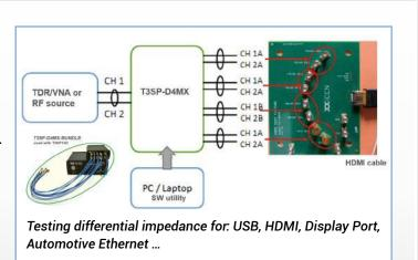
cables, there is always the possibility that even your premium cables may have some imperfections that can cause measurement artifacts. The T3SP-series TDR reveals immediately the quality of your multi-channels differential pairs cables and connectors, identifying parts that are out of spec, due to damage or defects. This drammatically improves your productivity and increases the confidence in your design and results.
