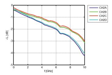
Insertion loss (IL) between CH1 or CH2-input and, respectively, CH1<X> or CH2<X> output ports.
