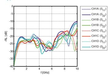
Return loss (RL) of CH1 and CH2-input (S11) when routed to 50  $\Omega$ -terminated output respectively CH1<X> port and CH2<X> port (S22).
