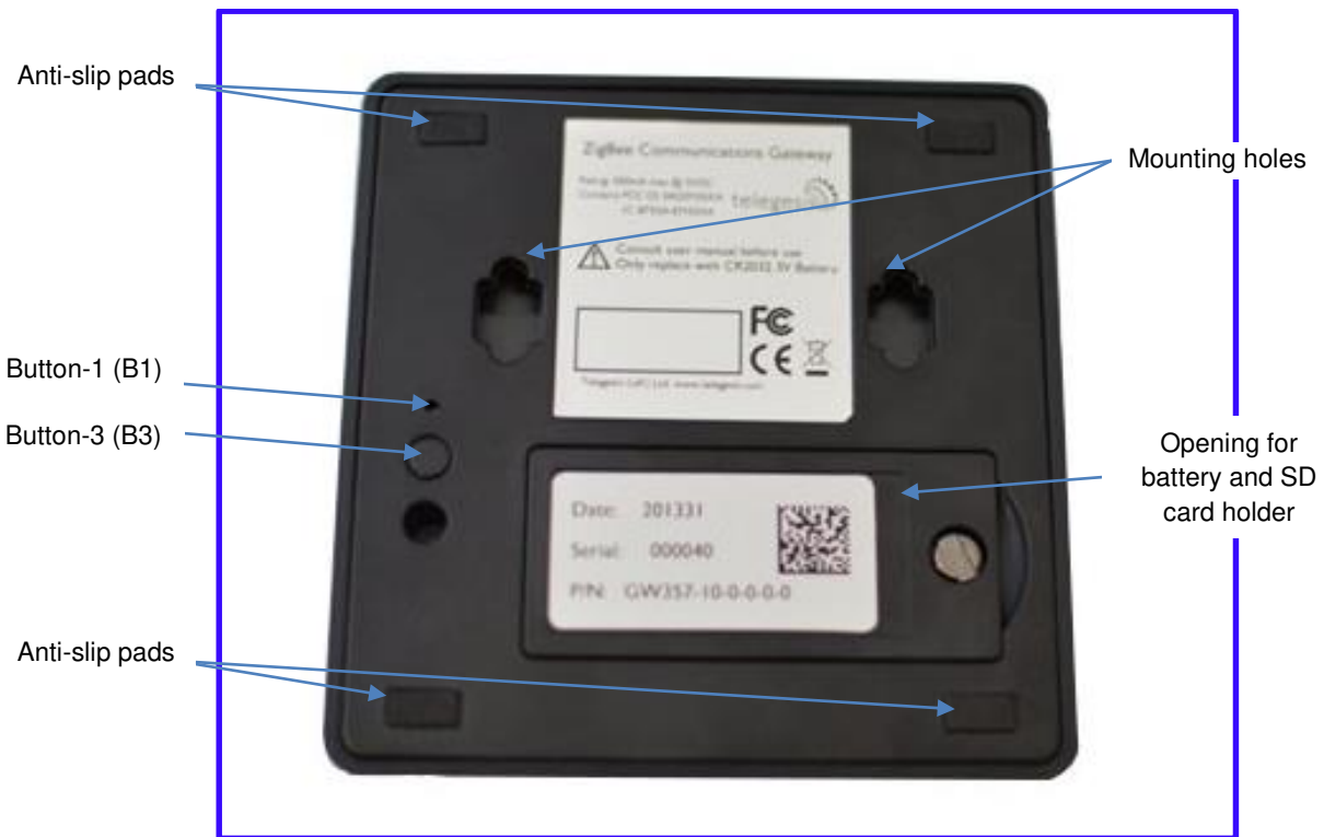
Figure 5: Gateway bottom view
