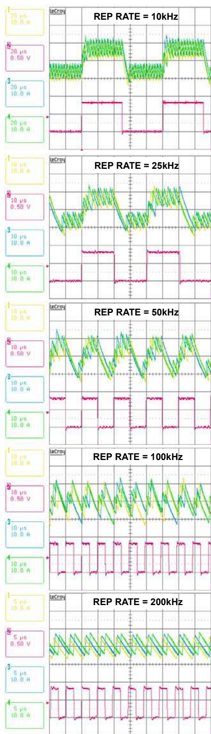
FIGURE 12. ISL62883 EVALUATION BOARD CURRENT BALANCING DURING DYNAMIC OPERATION. CH1: IL1, CH2: I LOAD , CH3: IL2, CH4: IL3
