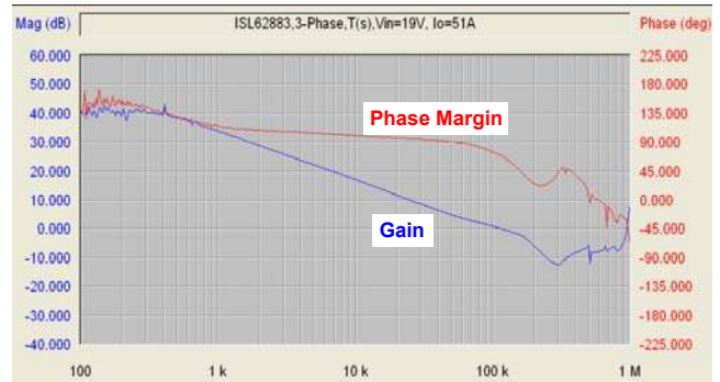
FIGURE 53. REFERENCE DESIGN LOOP GAIN T2(s) MEASUREMENT RESULT
