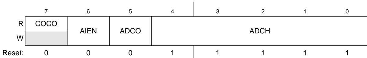
Figure 10-3. Status and Control Register (ADCSC1)
