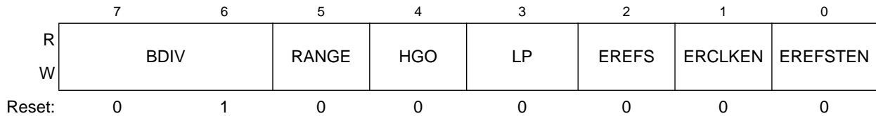
Figure 8-4. MCG Control Register 2 (MCGC2)
