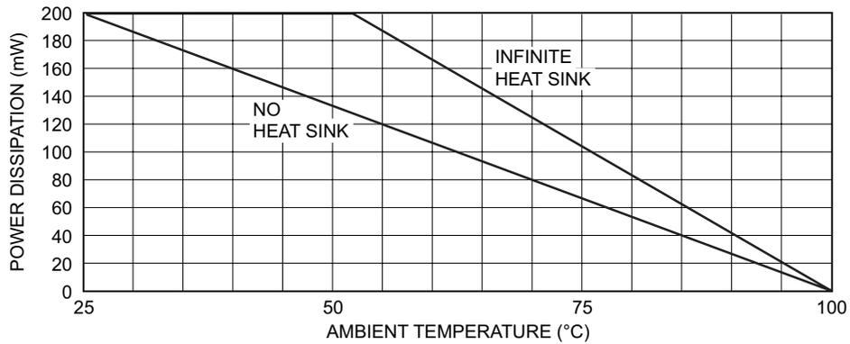
Typical Degradation Curve
