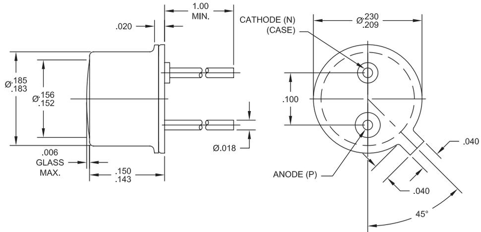
All surfaces are gold plated. Dimensions are nominal values in inches unless otherwise specified. Window caps are welded to the case.
