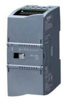
SIPLUS S7-1200 SM 1231 4AI based on 6ES7231-5ND32-0XB0 with conformal coating, -20...+60 °C, analog input, SM 1231, 4 AI, +/-10 V, +/-5 V, +/-2.5 V, +/-1.25 or 0-20 mA/4-20 mA, 15 bit+sign bit
