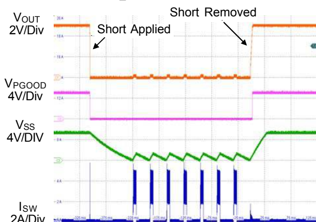
Figure 3. Short Circuit Protection and Recovery
