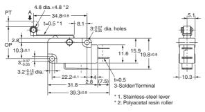
D2MV-1L2-1C3 Model Operating D2MV-01L2-1C3 characteristics Operating Force OF Max 0.29N {30 gf} Releasing Force RF Min. 0.02N {2 gf} (reference value) PT Max Pretravel 3.3 mm Overtravel OΤ Min. 2.1 mm Movement Differential MD Max 0.7 mm Operating Position OP 20.7±1.2 mm
