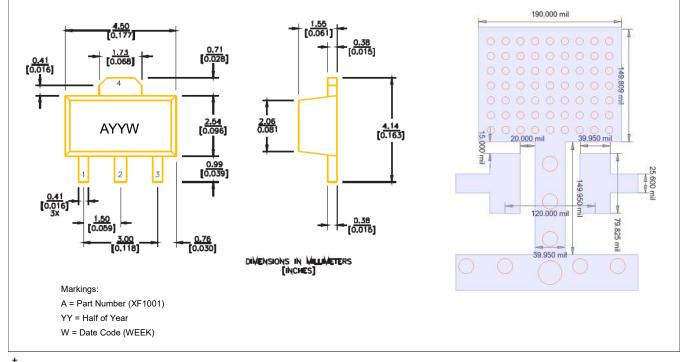
Reference Application Note M538 for lead-free solder reflow recommendations. Meets JEDEC moisture sensitivity level 1 requirements.
