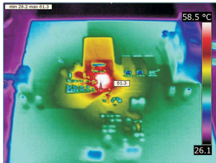
Figure 12. CSD86350Q5DEVM-604 Thermal Image
