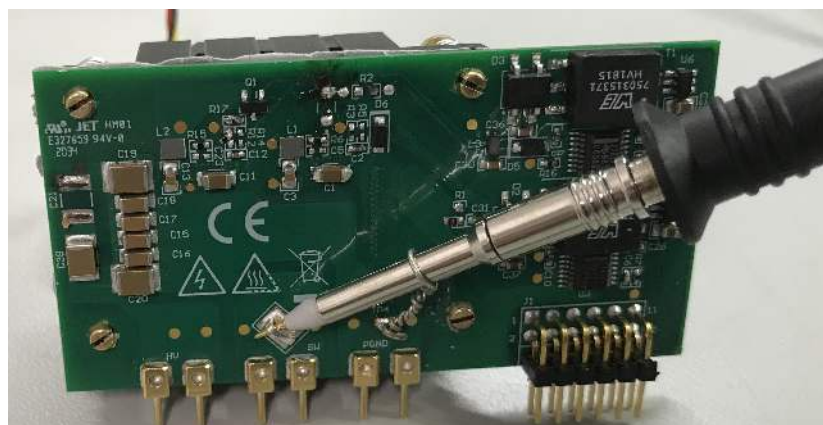
Figure 7-3. Switch-Node Voltage Measurement with High-Bandwidth Probe and Pigtail Ground Connection
