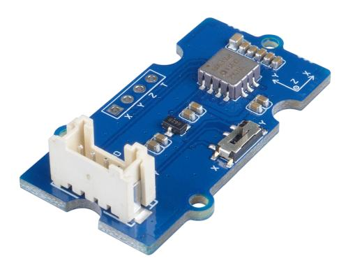
**Grove - 3-Axis Analog Accelerometer ±20g (ADXL356B)**
