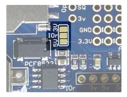
The IOREF pin should come from the Arduino main board being used.
