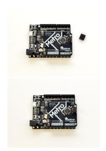
Place the 2x3 female header on to the Arduino/Metro
