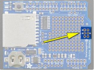
This is the "R3 compatible" Datalogger. Note that it has a smaller prototyping area and that there is a 2x3 SPI header spot on the right
