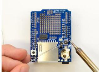
Flip around and solder the other side as well as the 2x3 header
