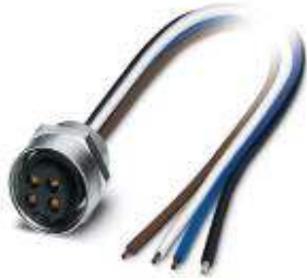
Sensor/actuator flush-type socket, 4-pos., 7/8", front mounting with Pg13.5 fastening thread, with 0.5 m PVC litz wire, 4 x 0.75 mm 2
