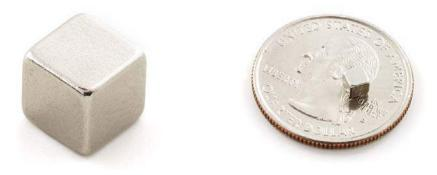
**Description:** These are very small rare earth magnets - 0.125" cubed. Composed of Neodymium/Iron/Boron (NdFeB), these magnets are curiously strong and make for a great way to attach tools to a metal workbench, hold small children to a fridge, and as a trigger for reed switches. Don't let the photo fool you - these are very small magnets.
