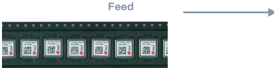
Figure 10: Orientation of NINA-B221 module on tape
