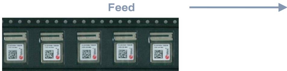
Figure 11: Orientation of NINA-B222 module on tape
