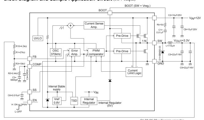
•C1,C8,C5,C9 = Ceramic capacitor •L1 = CDRH105RNP-100NC (sumida)
