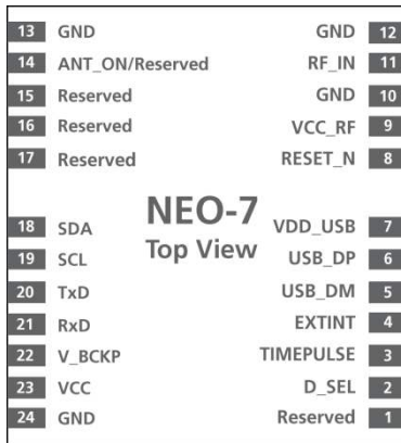
Figure 2: Pin Assignment
