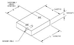
MELCOR's spacer blocks widen the gap between the cold surfaces and hot side heat exchanger, allowing for more insulation material. The spacer blocks are intended for use with our CP, PT, or HT series of thermoelectrics as part of a complete thermoelectric system.
