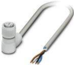
Sensor/Actuator cable, 4-position, PP-EPDM halogen-free, Gray RAL 7035, Free cable end, on Socket angled M12, A-coded, Cable length: 5 m, Hygienic design, with plastic knurl
