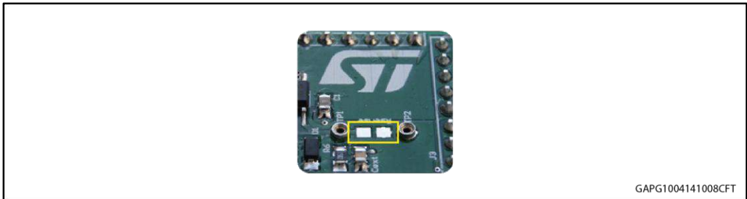
Figure 5: Pads for soldering SMD resistor
