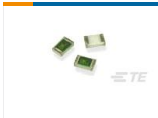
TE Part #1676385-2 RN 0805 5K11 0.1% 10PPM 1KRL
