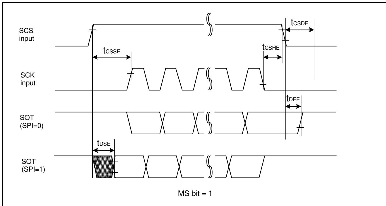
**High-Speed Synchronous Serial (SPI = 0, SCINV = 0)**
