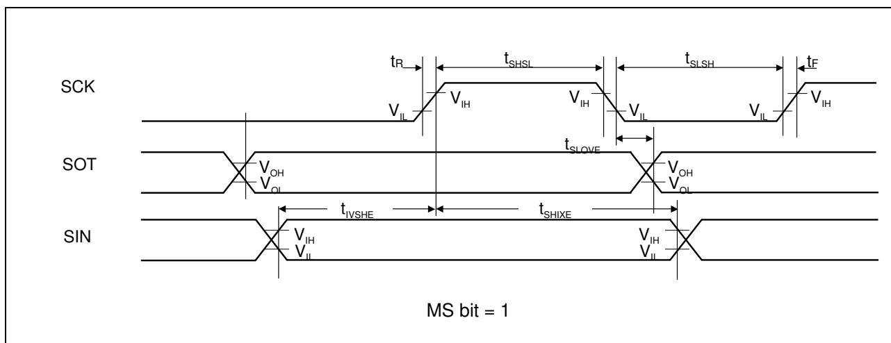
**When Using Synchronous Serial Chip Select (SCINV = 0, CSLVL=1)**
