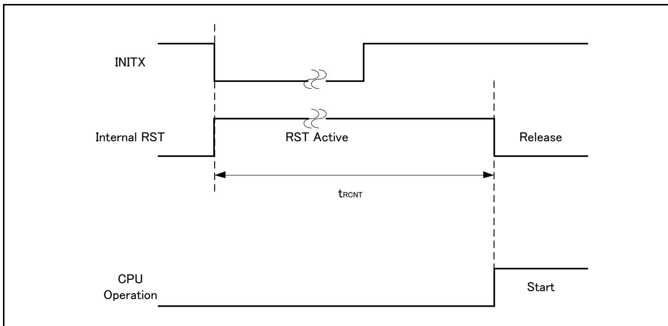
**Example of Standby Recovery Operation (when in Internal Resource Reset Recovery\*)**
