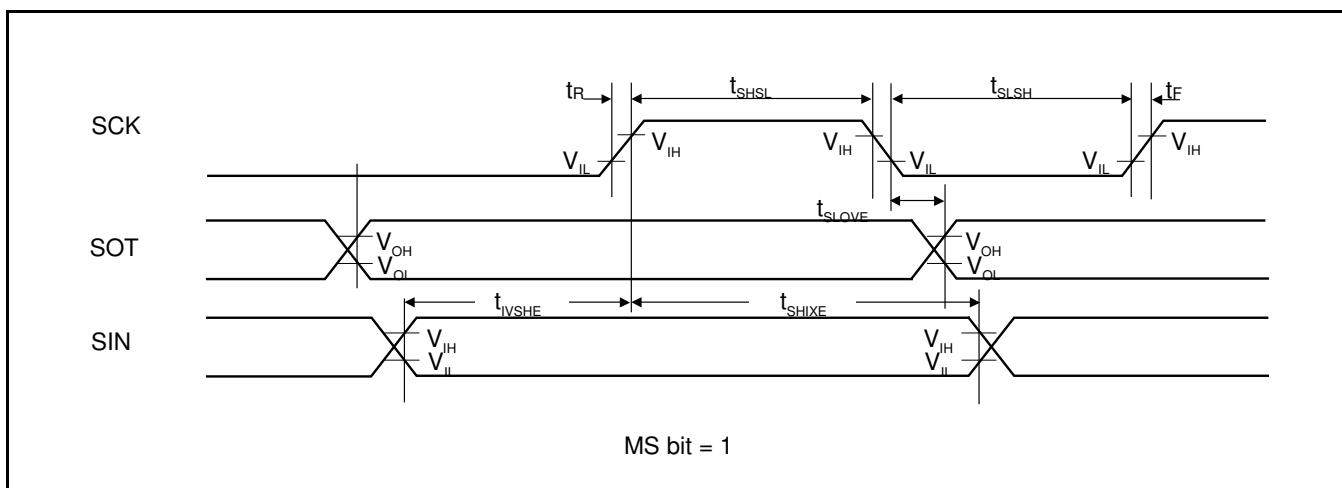
**When Using High-Speed Synchronous Serial Chip Select (SCINV = 0, CSLVL=1)**
