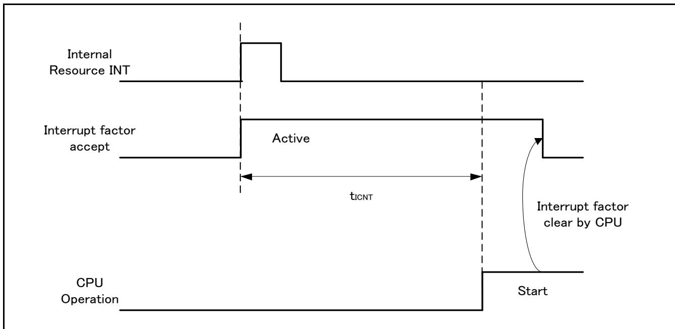
\*: Depending on the standby mode, interrupt from the internal resource is not included in the recovery cause.
