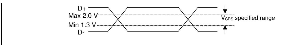
\*5: They indicate Rising time ( $t_{FR}$ ) and Falling time ( $t_{FF}$ ) of the Full-speed differential data signal.
