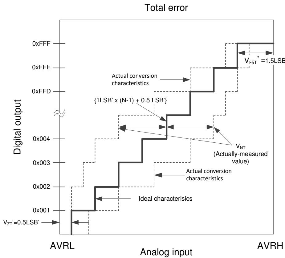
$$\text{Total error of digital output } N = \frac{V_{NT} - \{1 \text{ LSB}' \times (N-1) + 0.5 \text{ LSB}'\}}{1 \text{ LSB}'} [\text{LSB}]$$
