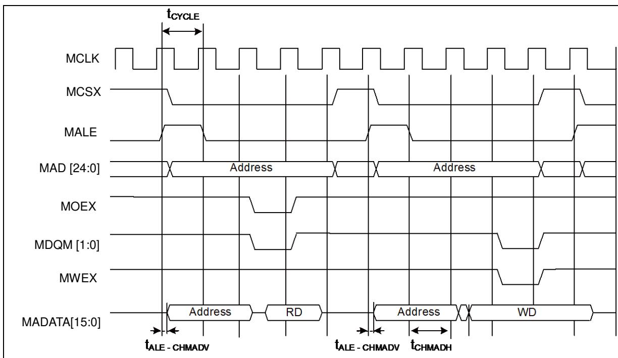
**Multiplexed Bus Access Synchronous SRAM Mode**
